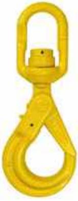
Austlift LS Type Swivel Self-Locking hook have a ball bearing swivel to allow the hook to swivel under load thus reducing the twist of a sling. Designed with enlarged eye for passing larger Shackles without disassemble of the hook.
