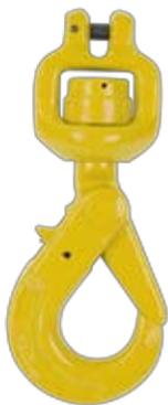
Austlift LT type Swivel Self locking hook, Clevis Type, fitted with a ball bearing which will allow the hook to swivel under load. The clevis type will let chain connected to the hook directly which makes the chain sling compact and friendly to use.
