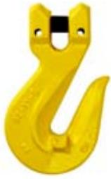
Austlift GC Type Clevis grab hook provides the flexibility to shorten Chain Slings and can be used for back-hooking. Austlift Grab Hooks come with supporting lugs to allow no reduction of the working load limit. The Clevis is designed for easy connection of Chain.
