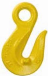
Austlift GE Type Eye grab hook provides the flexibility to shorten Chain Sling and can be used for back-hooking. Austlift Grab Hooks come with supporting lugs to allow no reduction of the working load limit. The eye is designed for easy connection of Chain Connector.
